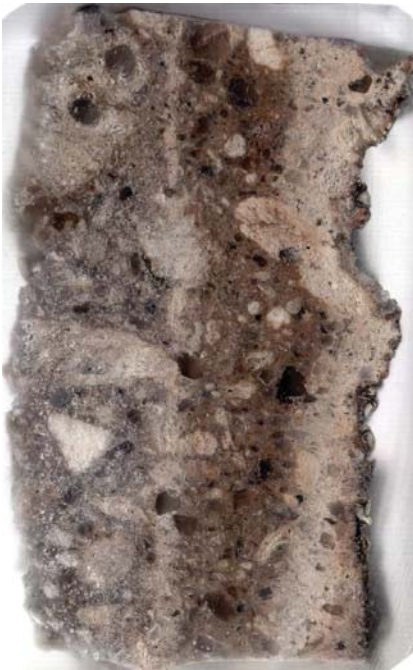
Fig. 16. Canyon-wall tuff with Type 7 alteration. The image is a thin section butt 2.5 cm wide cut perpendicular to the canyon wall. The canyon wall is on the right side of the image. The case hardened zone is made up of two parallel bands of alteration. The outer alteration band, next to the canyon wall, is mostly white in color. The inner alteration band ranges is medium to dark brown in color. Both bands are extensively altered, but the inner band is more highly mineralized. The tuff left of the inner band of alteration is slightly altered and contains abundant volcanic glass. Porosity is 20 to 30% in the outer band, 1 to 15% in the inner band, and 30 to 40% in the slightly altered tuff.
